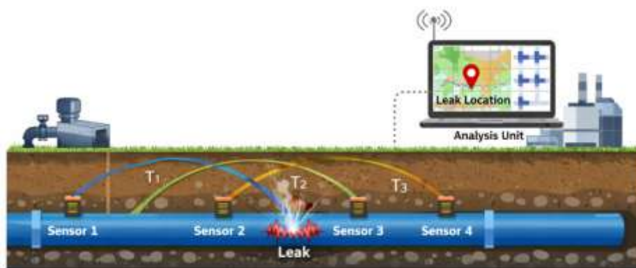
Figure 1: General illustration of an acoustic leak localization system using multiple sensors along a pipeline.
